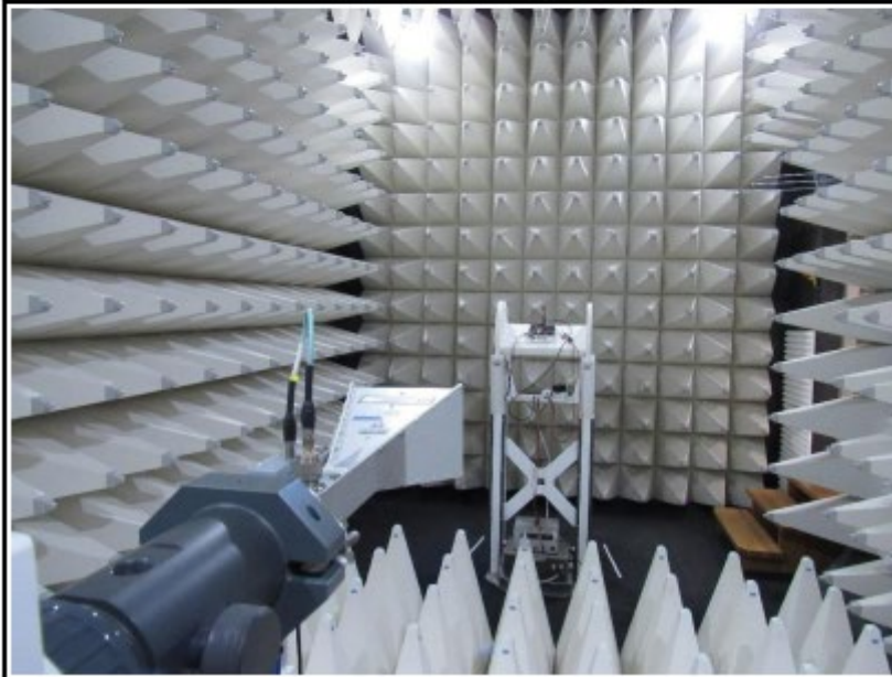
Setup for measurements above 1 GHz-Antenna 1
