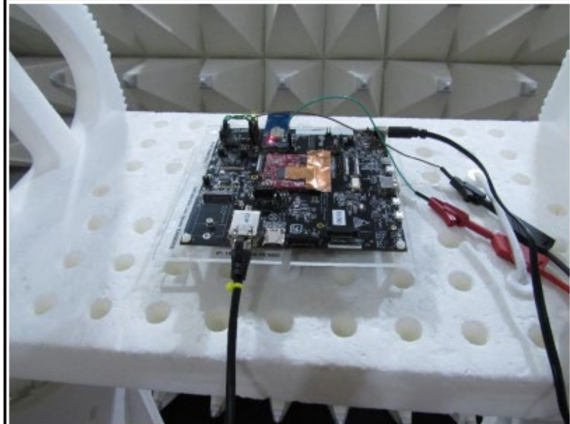
EUT Test Setup above 1 GHz-Antenna 3
