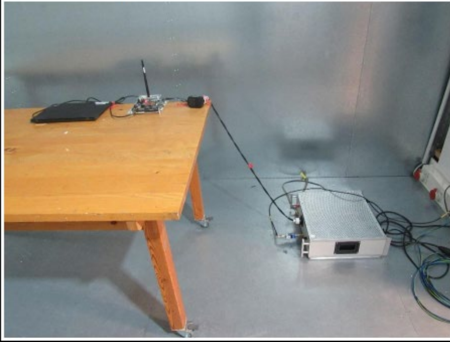
Setup for measurements 150 KHz - 30 MHz
