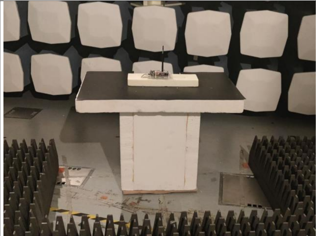
Picture14, Radiated Spurious Emissions, EUT setup, RX 1 – 12,75 GHz
