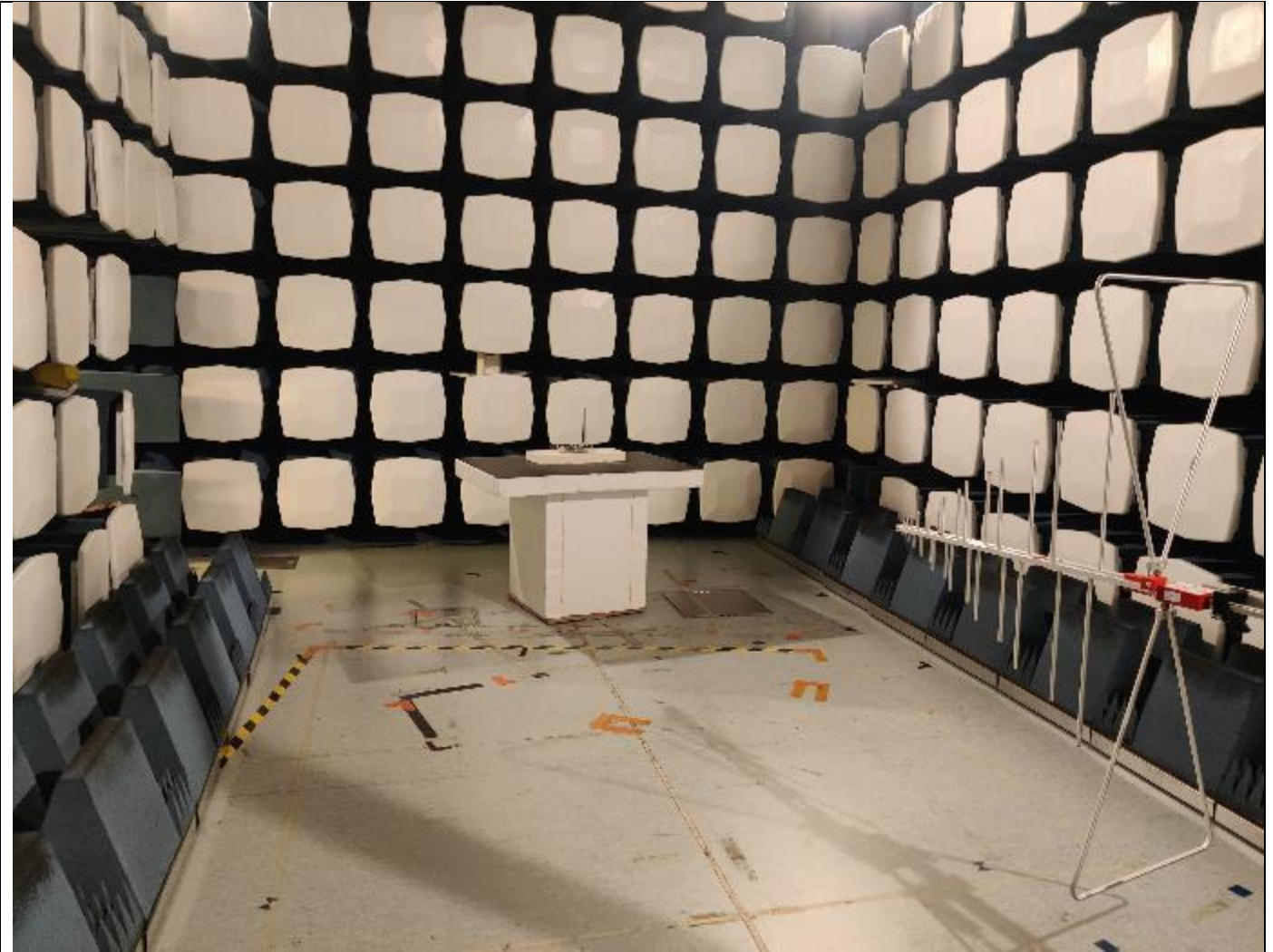
Picture 9, Radiated Spurious Emissions, common setup, TX and RX 30 - 1000 MHz
