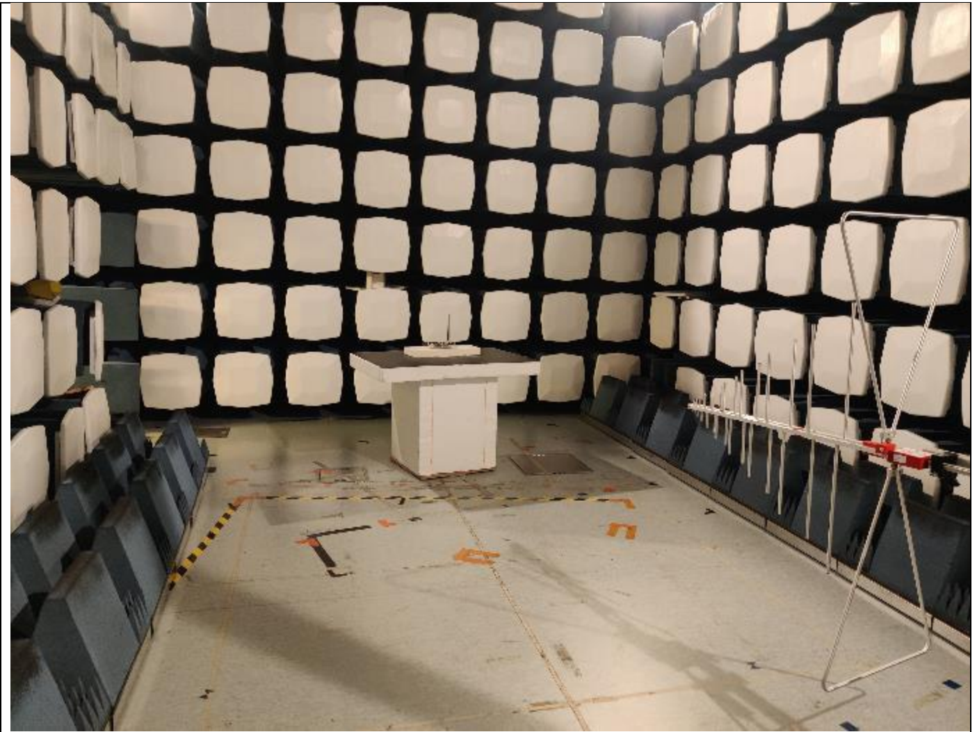
Picture 8, Radiated Emissions, common setup, 30 - 1000 MHz
