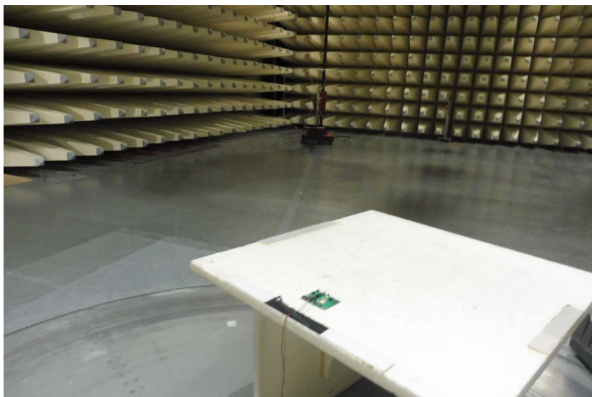
Photo 8: EUT at the semi-anechoic chamber
