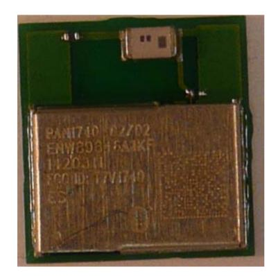
The above picture shows the full module with the case. The laser marking is made on the whole case.
