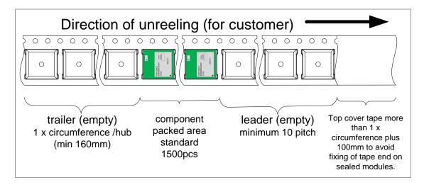
Empty spaces in the component packed area shall be less than two per reel and those spaces shall not be consecutive.
