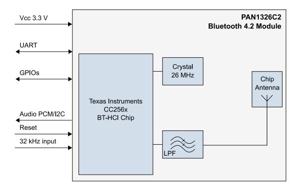
The Slow Clock 32.768 kHz is mandatory, otherwise the module does not start up  $\Rightarrow$  2.4 Clock Inputs.
