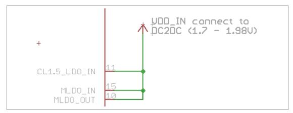
Mixed DC2DC-V<sub>BAT</sub> system (Maximum RF output power and optimum system power, but requires routing of  $V_{BAT}$ :
