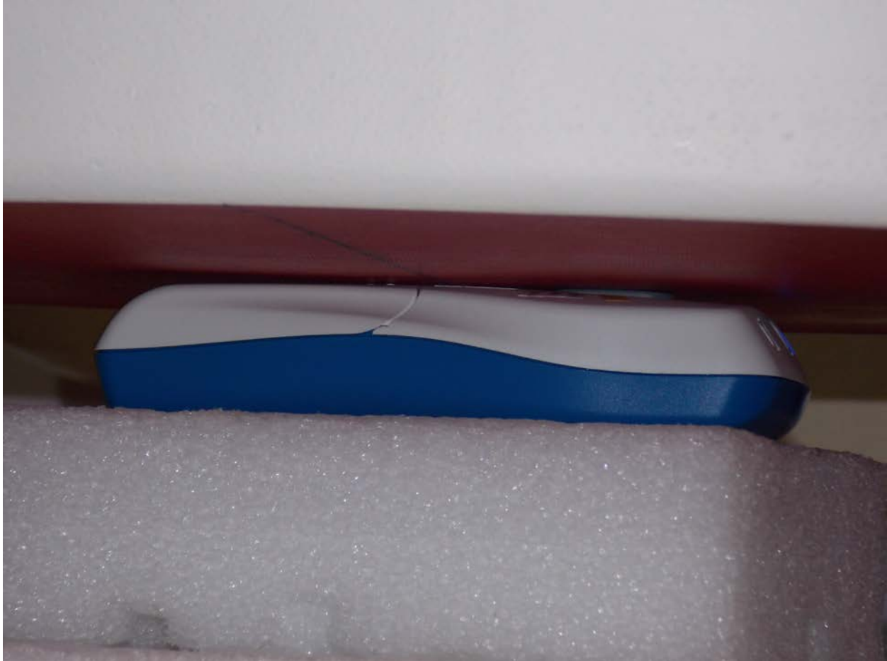
Test Position Front 0 mm Gap
