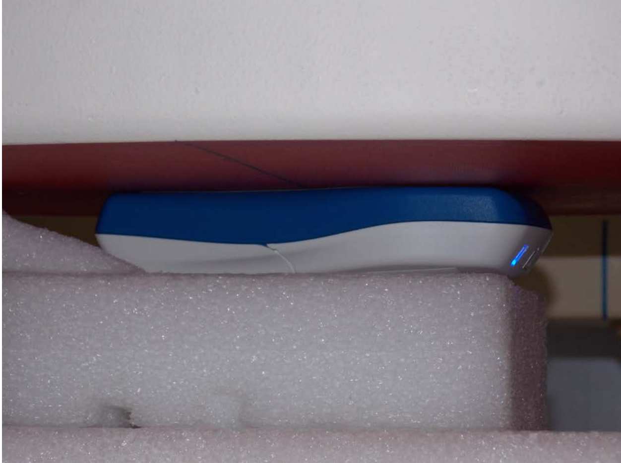
Test Position Back Face 10 mm Gap
