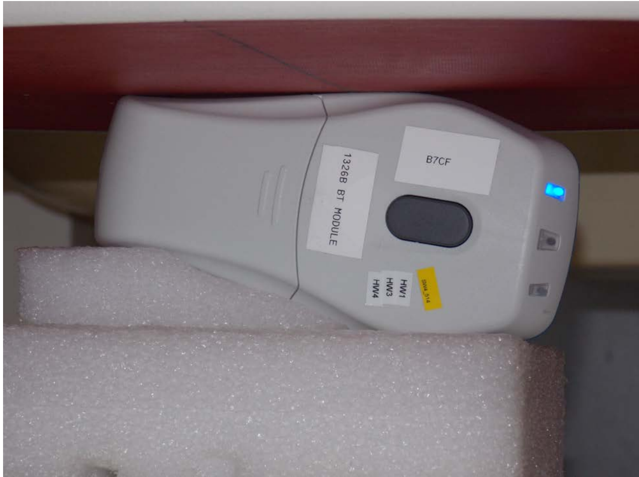
Test Position Left Side Body 0 mm Gap
