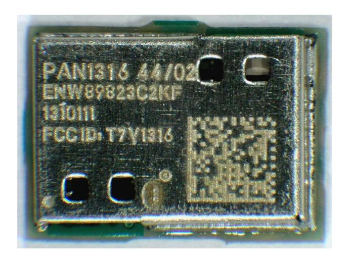
The above picture shows the full module with the case, the laser marking is made moreless on the whole case.
