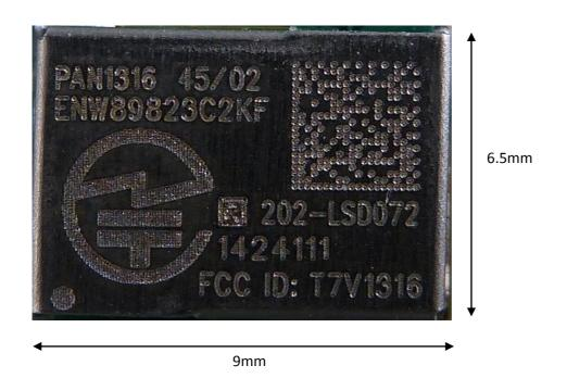
The above picture shows the full module with the case, the laser marking is made more or less on the whole case. Therefore the IC ID can not be placed on the label. The 2D code area can not be used. The IC 216Q-1315 is listed in the user manual only.
