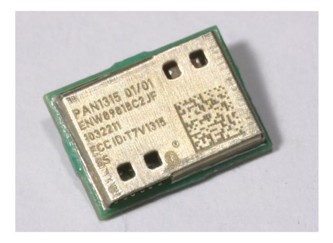
The above picture shows the full module with the case, the laser marking is made moreless on the hole case.
