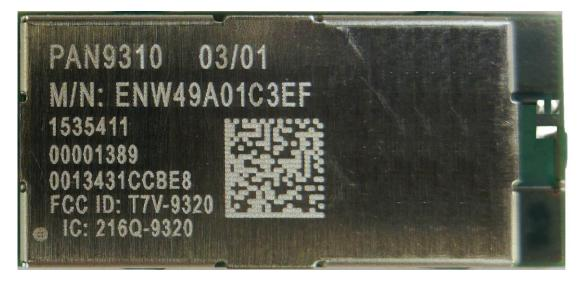
The above picture shows the full module with the case. The laser marking is made more or less on the whole case.
