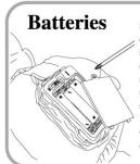
3 AA batteries are included for demonstration purposes and may need to be replaced by consumer. Alkaline batteries are recommended. To replace batteries, use Phillips screwdriver to loosen screw on battery compartment cover. Lift cover and replace batteries. Once batteries are replaced, close cover and tighten screw.
