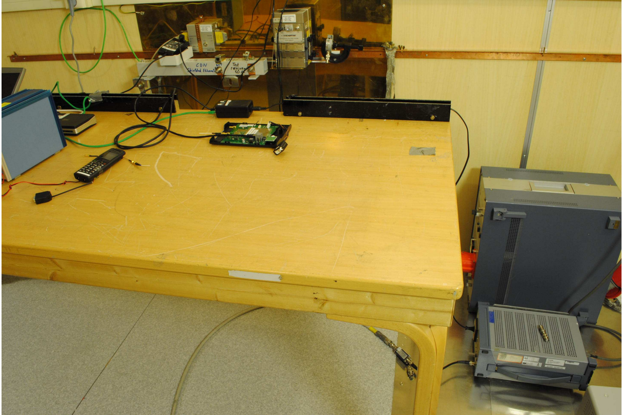
Power line Conducted Emissions Test Set-up
