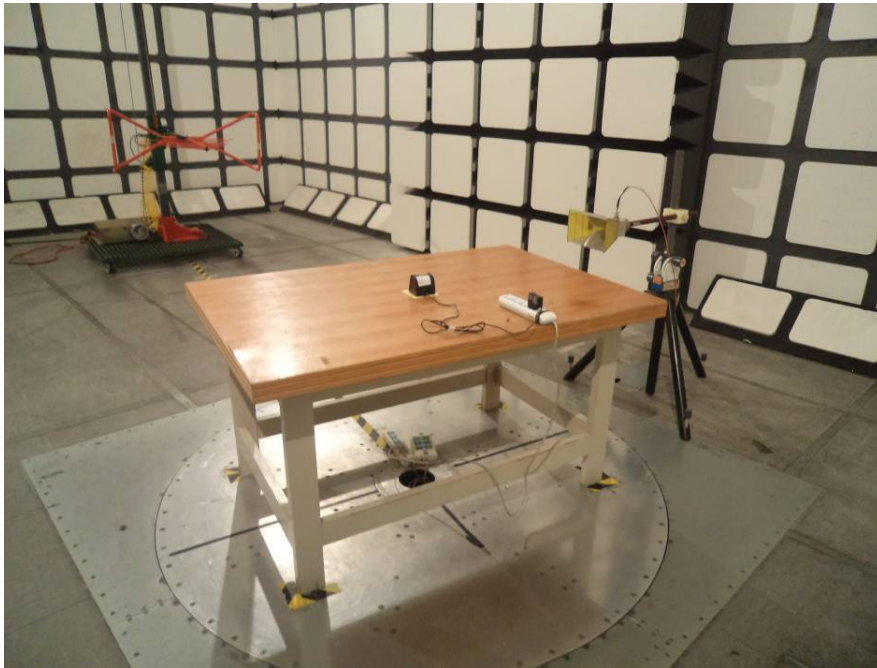
Radiated Emissions View (Below 1 GHz)
