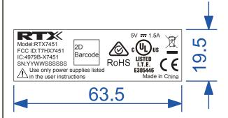
SIZE : W63.5mm x H19.5mm MATERIAL : PET COLOR : Black text on white background POSITIONING : Affix on the base bottom
