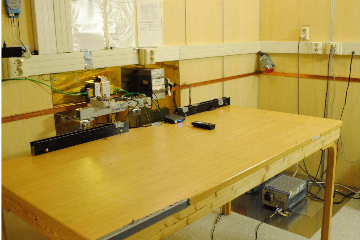
Power line Conducted Emissions Test
