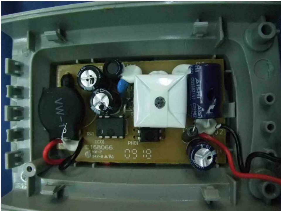
Telephone Line Extender another Main PCB comp side
