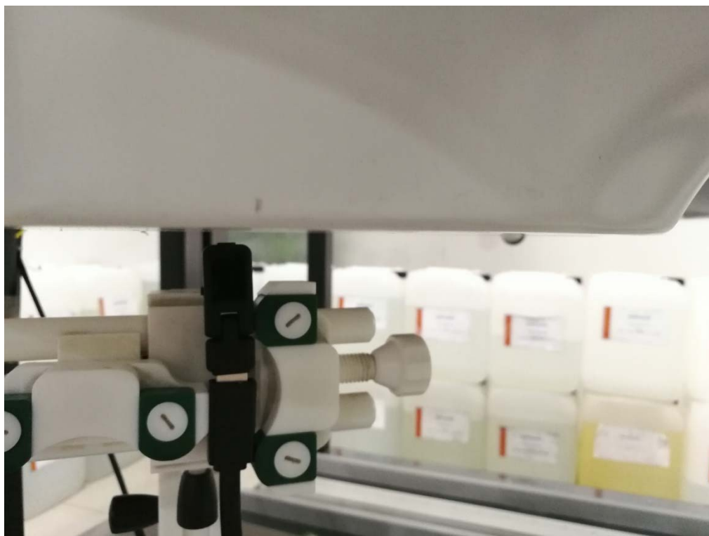
Body Top Edge (separation distance is 5mm)
