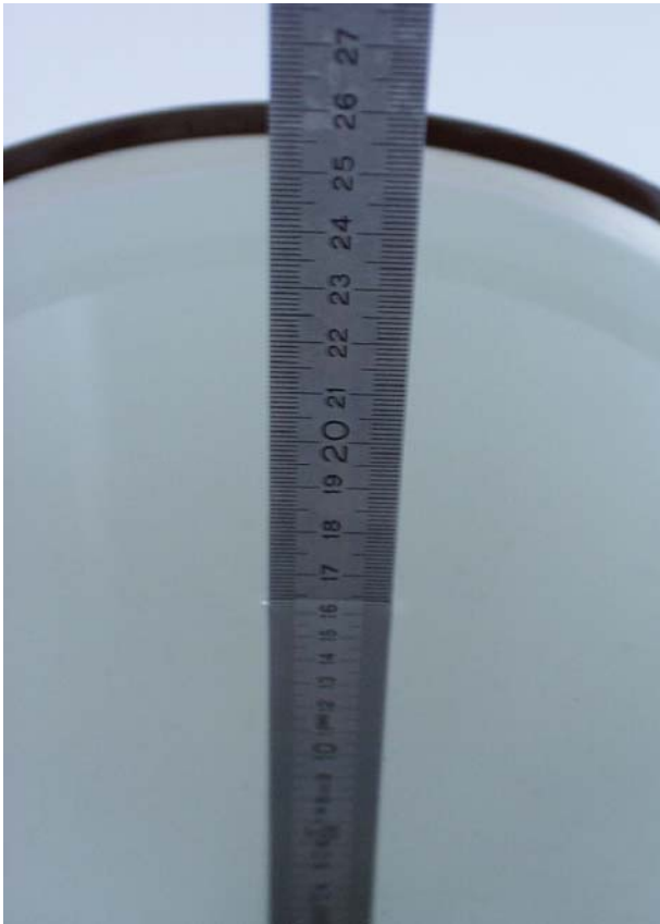
Fig. 22: Liquid depth for 1900 MHz Head measurements
