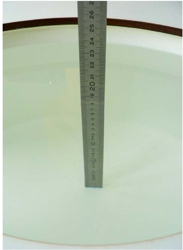
Fig. 23: Liquid depth for 1900 MHz Body worn measurements
