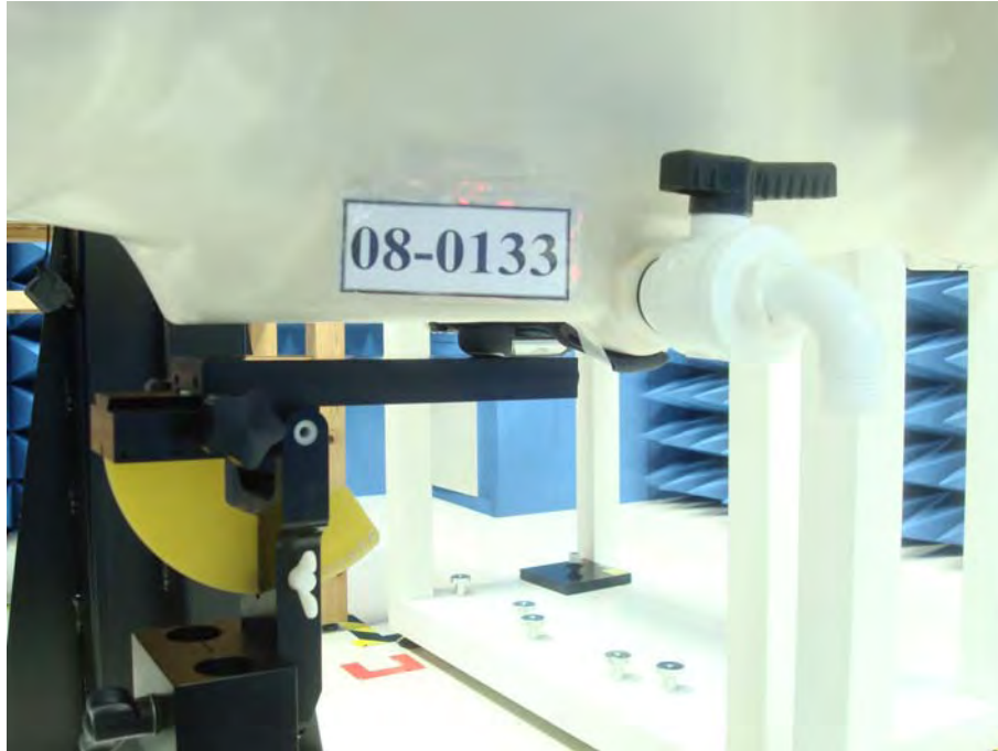
Figure 12. Body SAR Test Setup _ Bottom to Phantom (0mm space)
