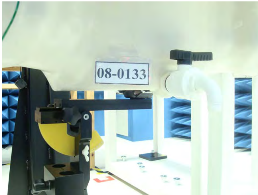
Figure 13. Body SAR Test Setup _ Top to Phantom (0mm space)
