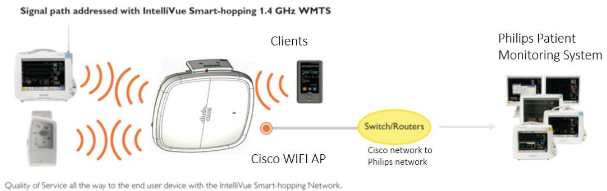
Figure.1. The RTX3300 Smart-hopping USB Access Point in the IntelliVue Smart-hopping network.
