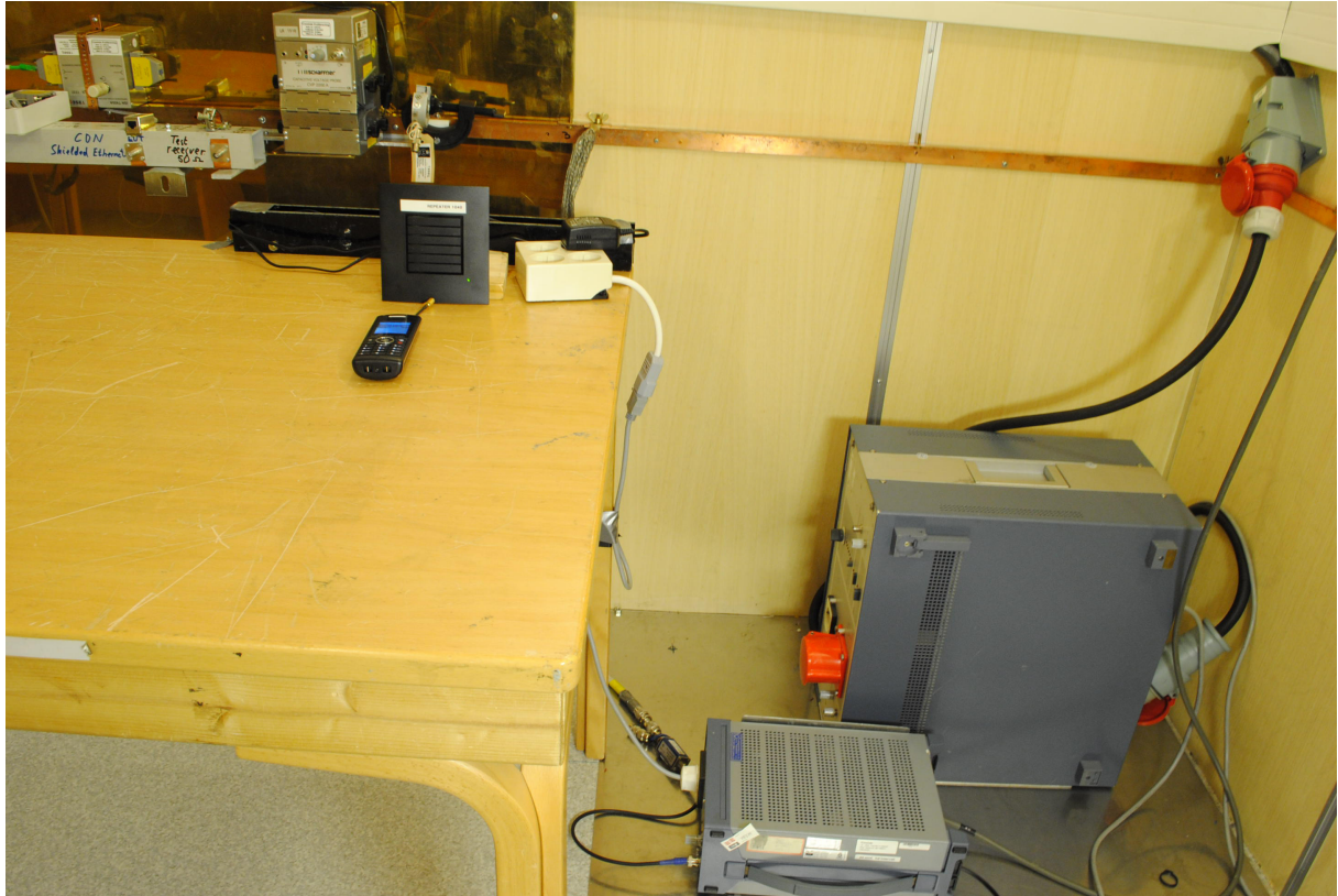
Power line Conducted Emissions Test Set-up
