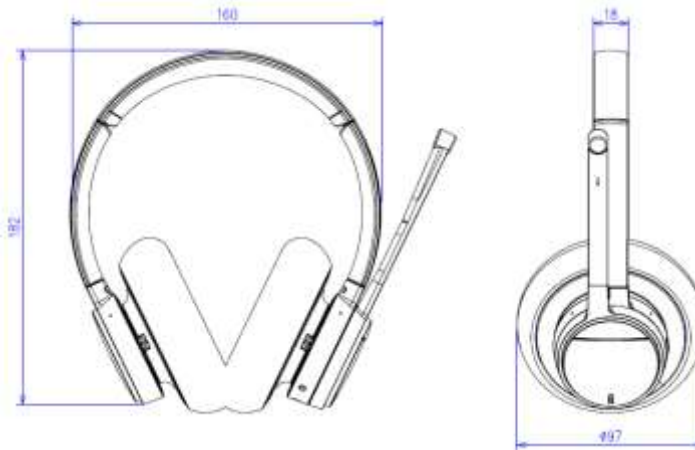
Fig.7: Dimensions of RTX7254
