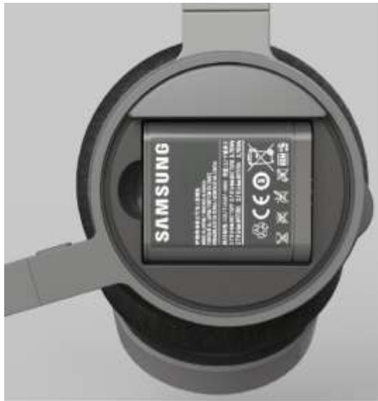
Fig.14: Battery lid removed
