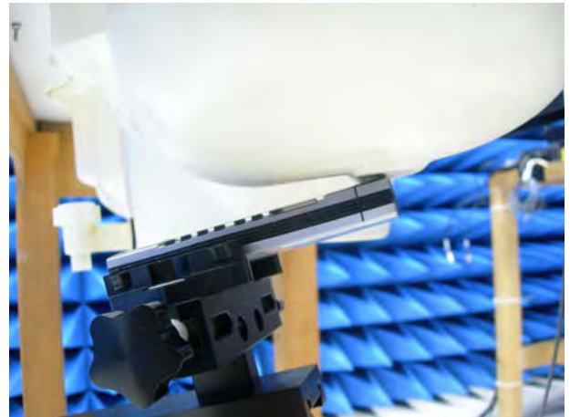
Figure 18. Left Head SAR Test Setup (Tilted)
