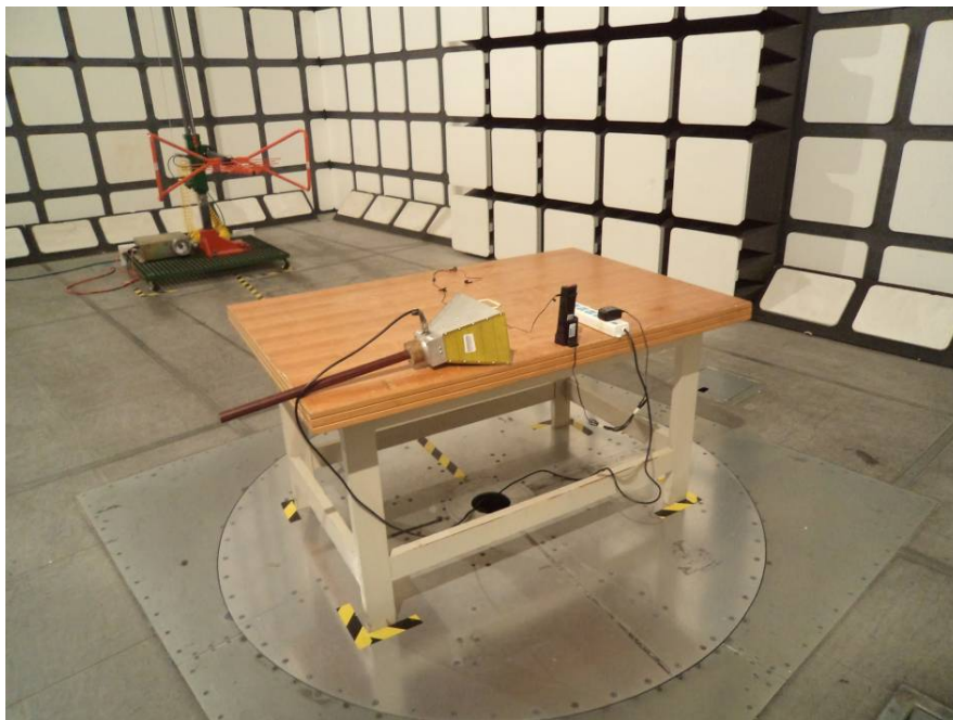
Radiated Emissions – Rear View (30-1000 MHz)
