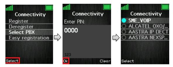
With this feature it is possible to connect the handset to another PBX than the one used by the base station system. In this way, the handset can for example function on a PBX without being connected to a system of base stations.
