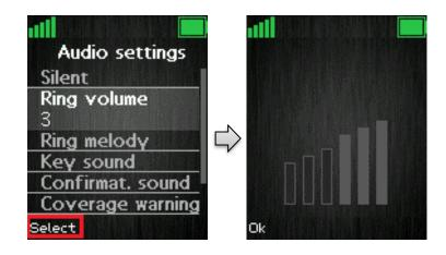
To select the desired ring volume the navigation keys up/down or right/left are used to respectively increase or decrease the volume. Thereby, pressing "Ok" saves the current ring volume. The currently applied ring melody is played when adjusting the ring volume so that the respective ring volume can be heard before selected.
