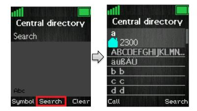
**NOTE:** When the central directory is in LDAP mode pressing right softkey "Back" the handset will return to the "Search" field, and a new search for a contact can be made. Pressing the red "On-hook" button, in the central directory, will send the user back to idle.
