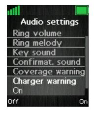
When the feature "Charger warning" is enabled (On), then an audible indication will be given when the handset is correctly connected to the charger. If the feature is set to "Off" no audible indication will be given when the handset is put in the charger.
