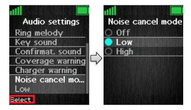
Noise reduction is a function used when the handset is in call. During a call, if noise reduction is enabled on the handset, the background noise around the user is reduced. In this way, the user should sound clearer to the counterpart since the background noise is reduced to a minimum.
