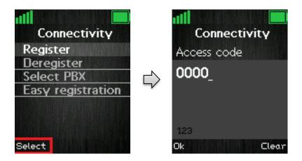
The access PIN code is default "0000" and cannot be changed via the handset. The access PIN code can only be changed via the web interface on the base (please check the additional document via [2] for more information about handset registration on a base system).
