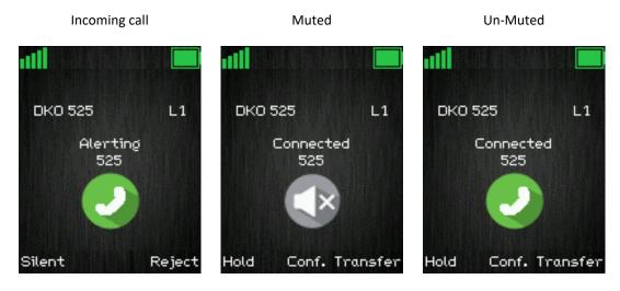
When the mute function is enabled during a call it is indicated on the "Connected" screen with the image shown above. Mute is turned off by pressing the mute button again.
