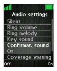
When the function "Confirmation sound" is enabled (On), an audible indication is given when an event succeeds or fails. For example, a positive confirmation sound is generated when a new setting is set or an entry is saved successfully in the phonebook. A negative confirmation sound is generated if the action fails. When the confirmation sound is set to "Off" no sounds are generated in either case.
