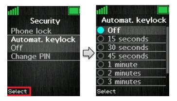
A list of selectable timeouts is displayed when the user enters the "Automatic keylock" menu. Any one of these can be selected by pressing the left softkey "Select" when the desired time interval is highlighted. Afterwards, when the handset has been inactive in the selected time interval the keypad will lock automatically.
