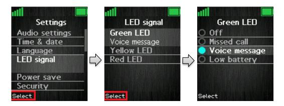
As seen in the images above each color of the LED signal (green, yellow, and red) can respectively be configured to indicate:
