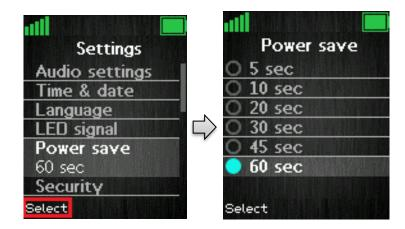
In the images above, it is displayed how the power save can be set between 5 seconds and 60 seconds. A certain time interval is chosen by pressing the left softkey "Select" when the desired time interval is highlighted.
