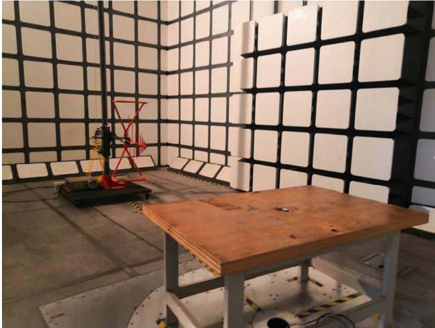
Radiated Emissions View (Below 1 GHz)
