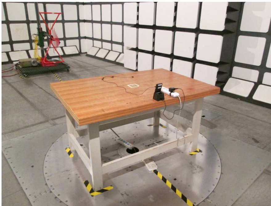
Radiated Emissions – Rear View (30-1000 MHz)
