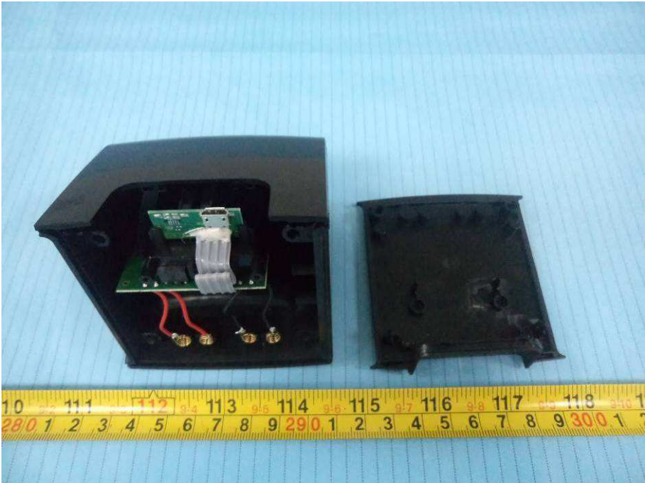
EUT (Charger) – Cover off View
