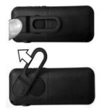
If the belt clip is installed, you must lift it up and maintain it in this position during the battery installation or replacement. You can also turn the belt clip counterclockwise.
