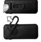
If the belt clip is installed, you must lift it up and maintain it in this position during the battery installation or replacement. You can also turn the belt clip counterclockwise. Lift up the cover.
