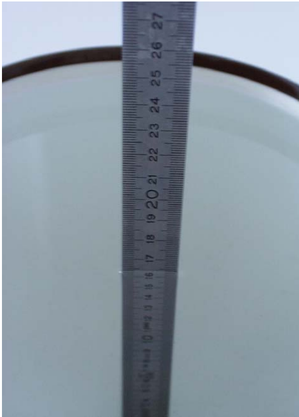
Fig. 22: Liquid depth for 1900 MHz Head measurements
