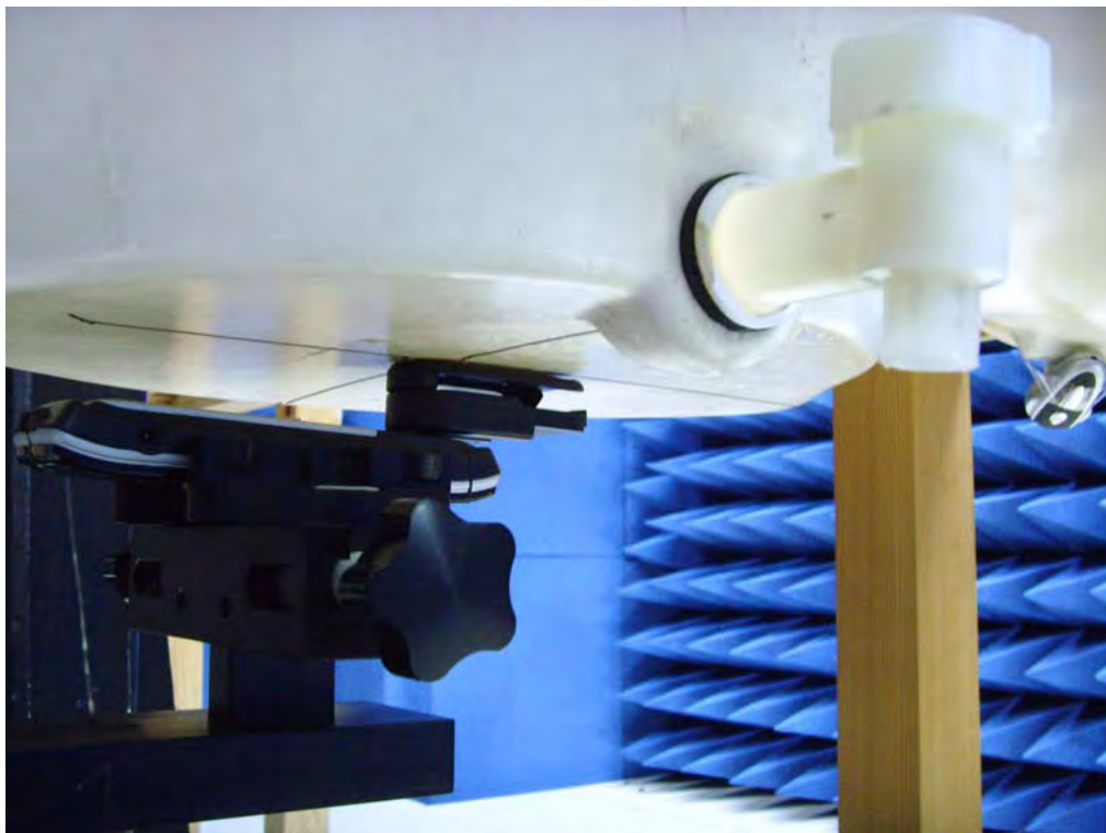
Figure 28. Body SAR Test Setup_ Bluetooth_ Headset_ Belt clip_2 (Flat Section)
