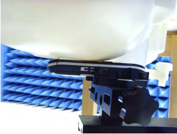
Figure 19. Right Head SAR Test Setup (Cheek)
