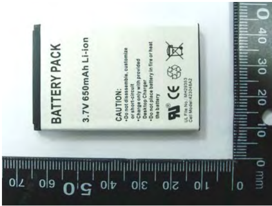
Figure 2. Battery (Li-ion 3.7V , 650mAh)
