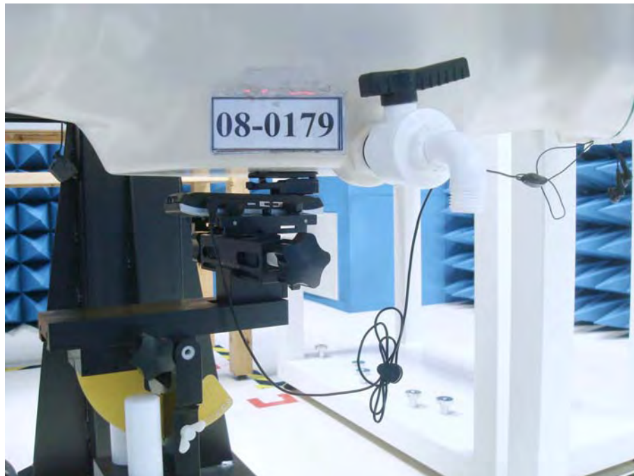
Figure 22. Body SAR Test Setup _ Back to Phantom with Headset & Belt Clip NO.2
