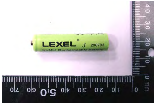
Figure 3. Battery (Ni-MH 1.2V , 600mAh * 3 PCS)
