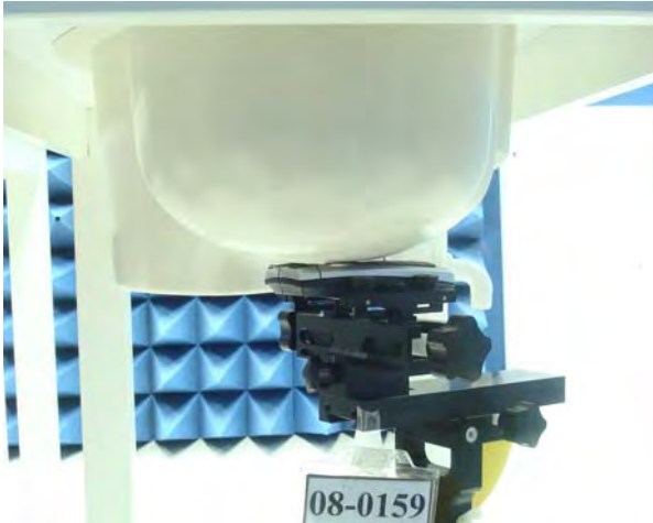
Figure 14. Right Head SAR Test Setup (Cheek)
