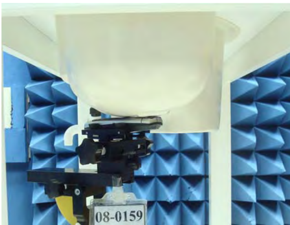
Figure 16. Left Head SAR Test Setup (Cheek)
