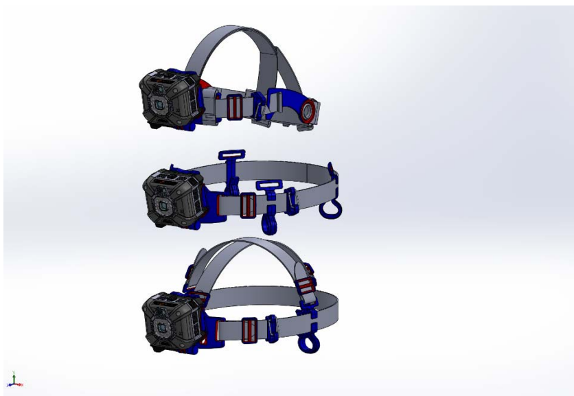
Figure 2. Mounting Variations: Headband, Hardhat, Climbing Helmet (top to bottom)
