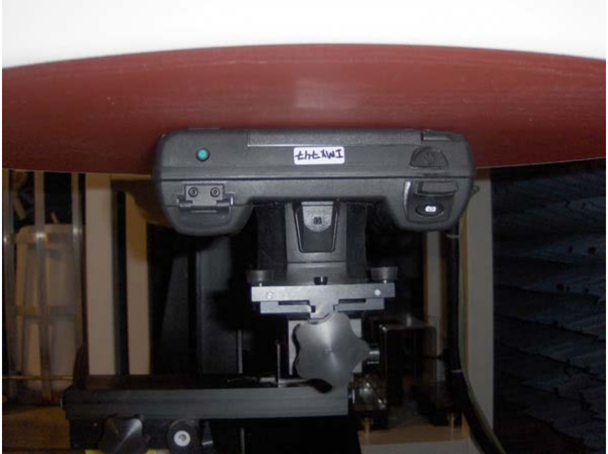
< Back-Touch working at 2.45GHz Band >
