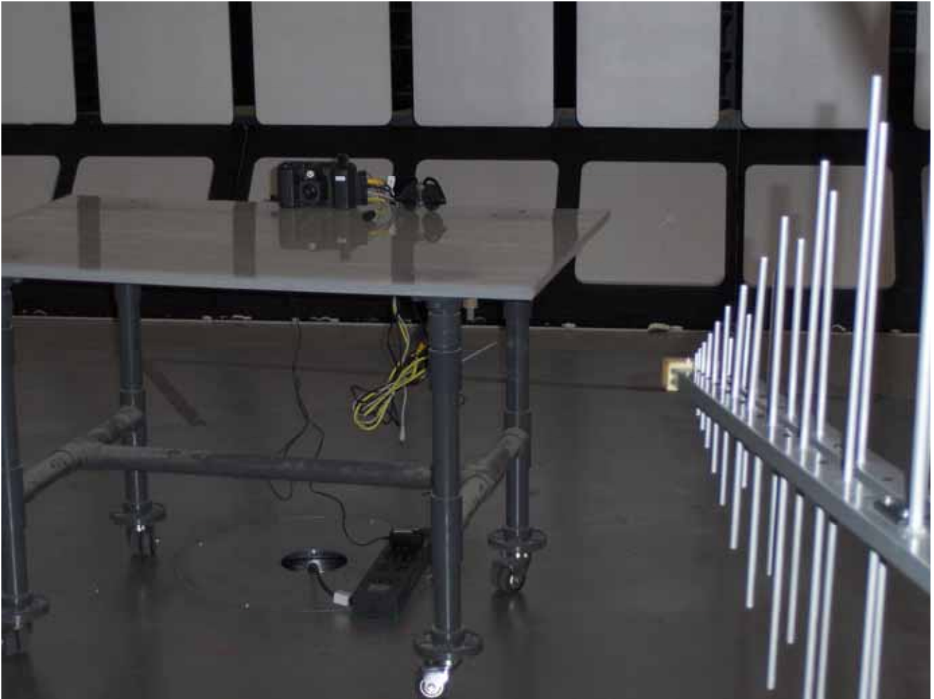
Radiated Emissions at 3 m Distance
