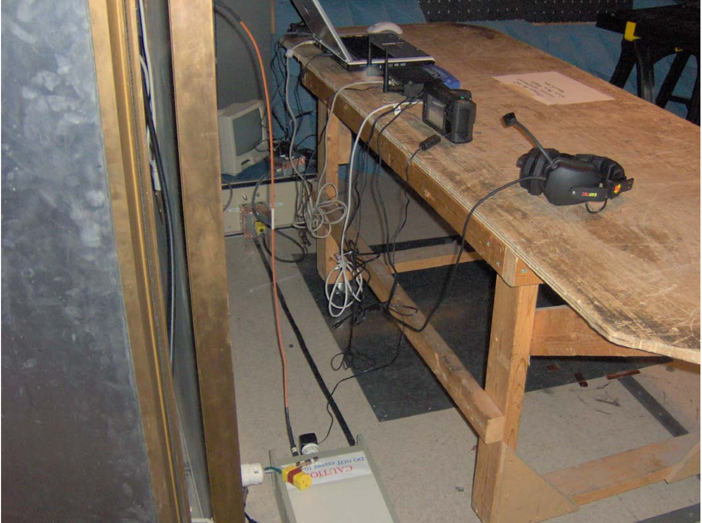
Photo #2: Test Setup for AC Powerline Conducted Emissions
