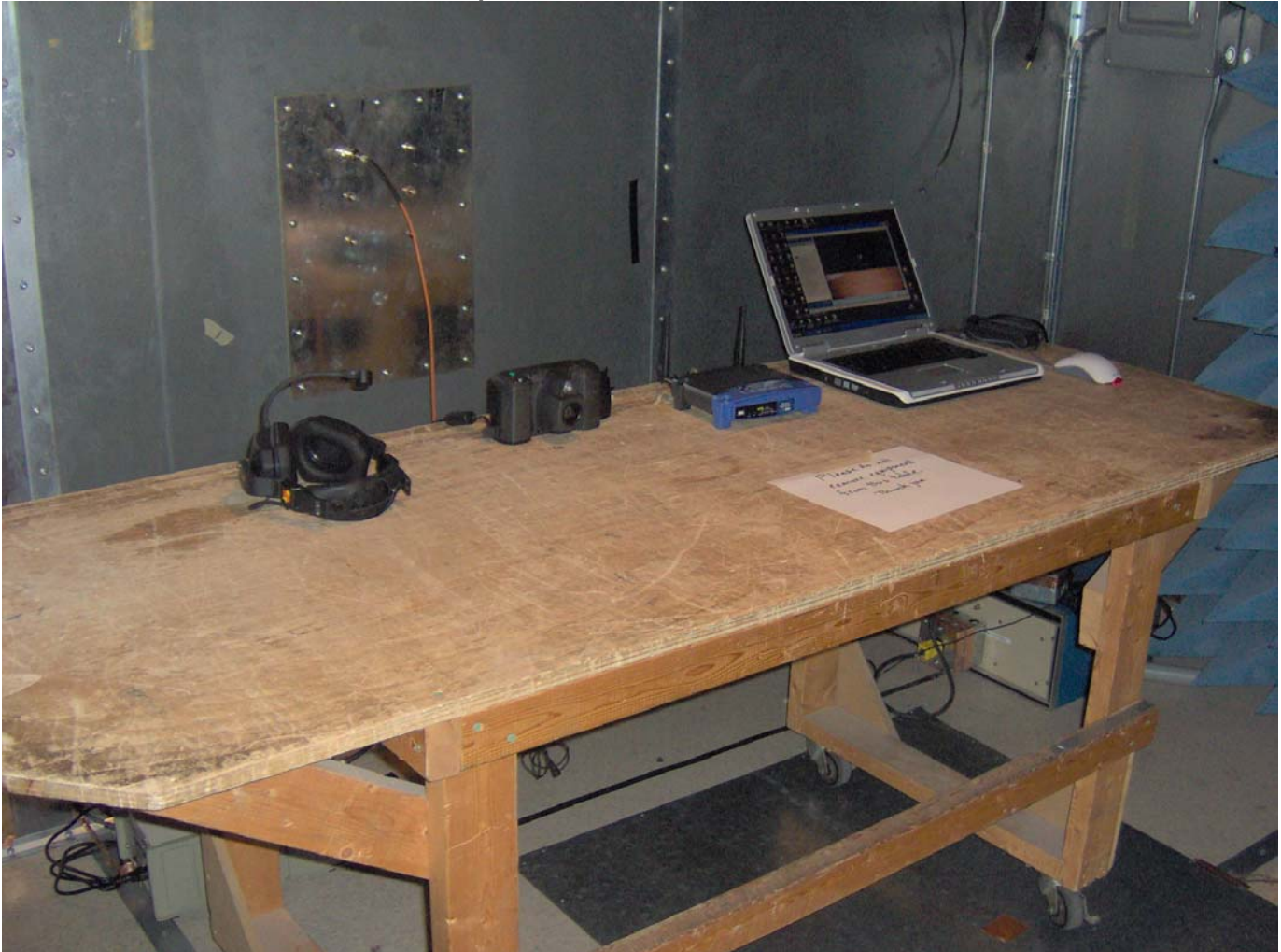
Photo #1: Test Setup for AC Powerline Conducted Emissions
