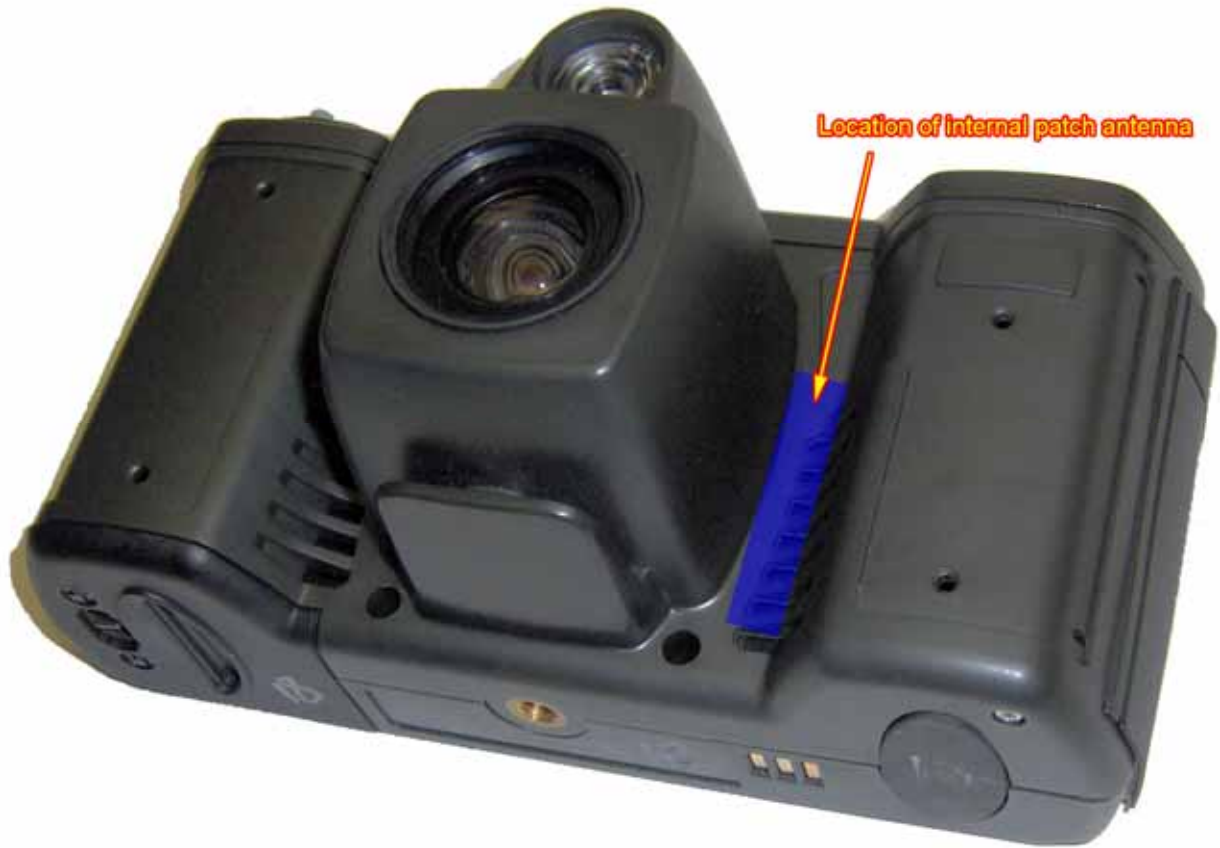
< Location of the internal patch antenna >
