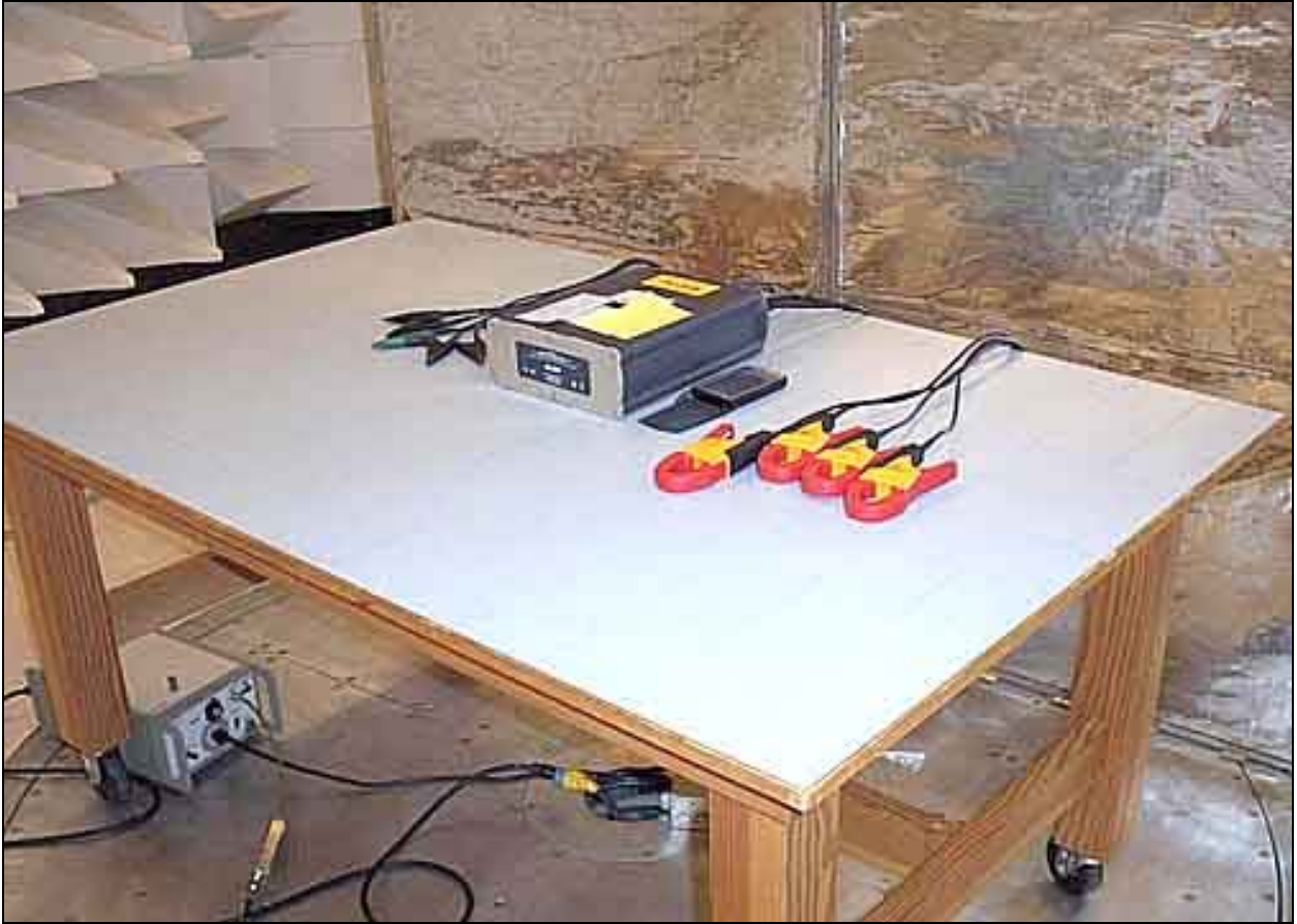
Mains Conducted Emissions - Front View
