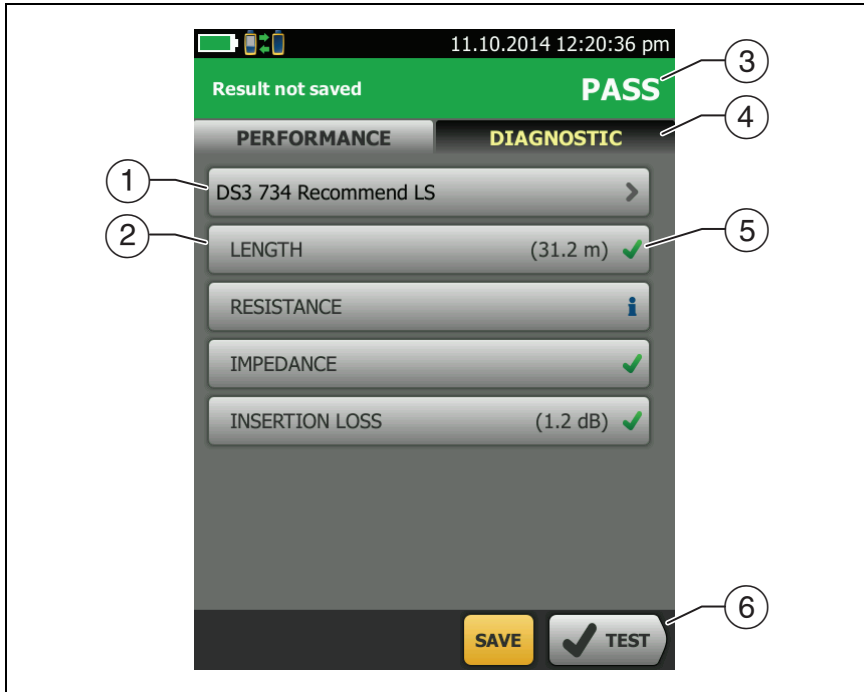
Figure 29. Autotest Results for Coaxial Cabling
