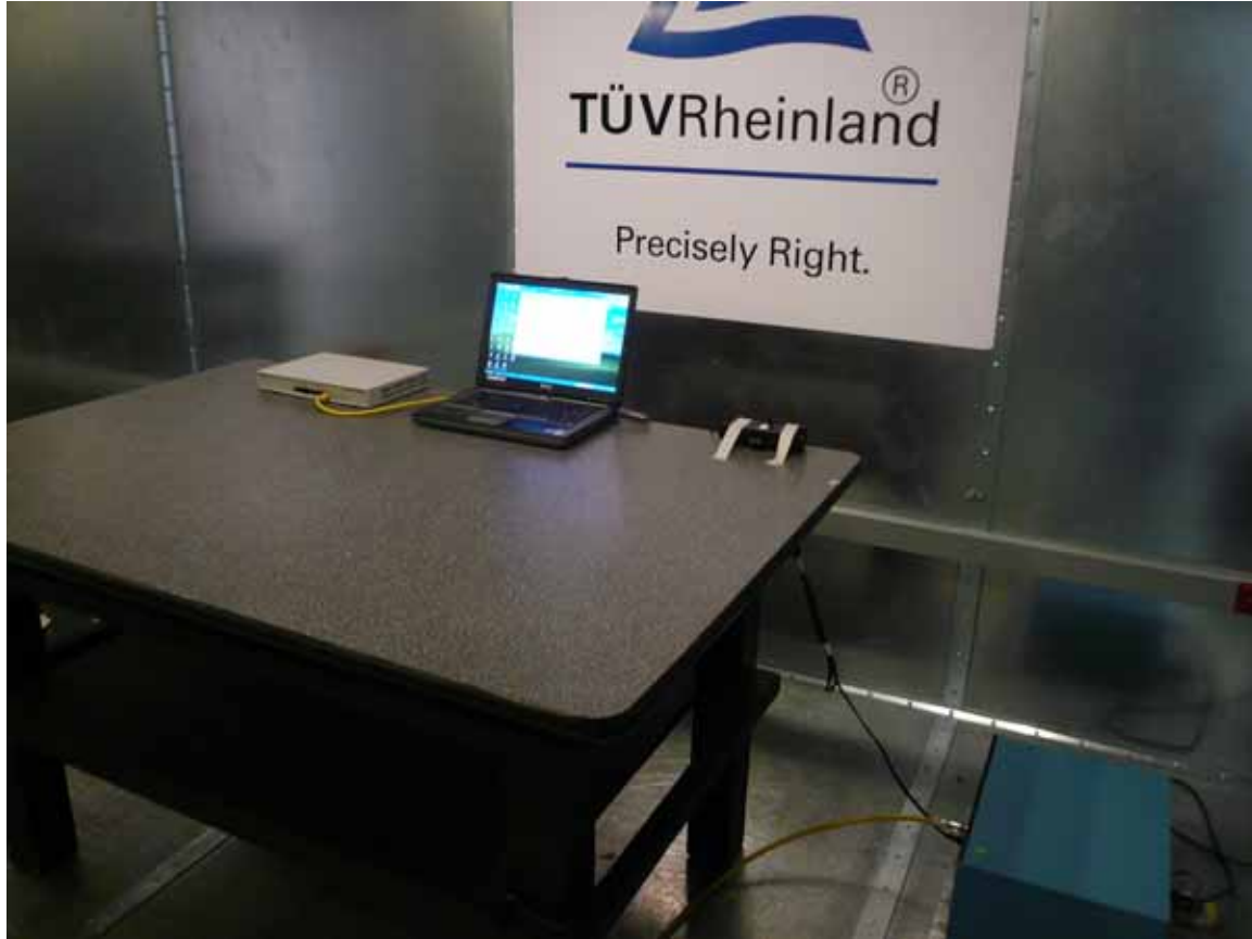
Figure 8: AC Conducted Emission Test Setup (Front)
