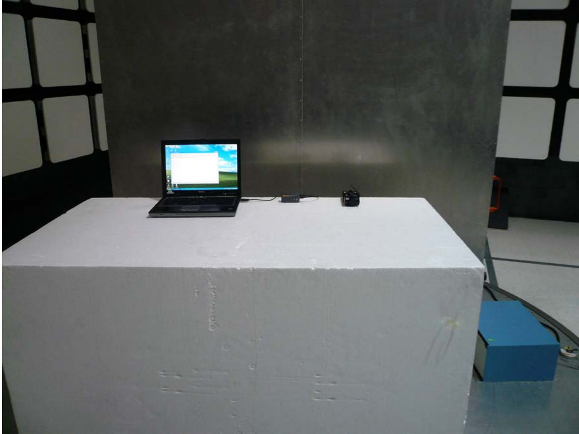
Figure 8: AC Conducted Emission Test Setup (Front)
