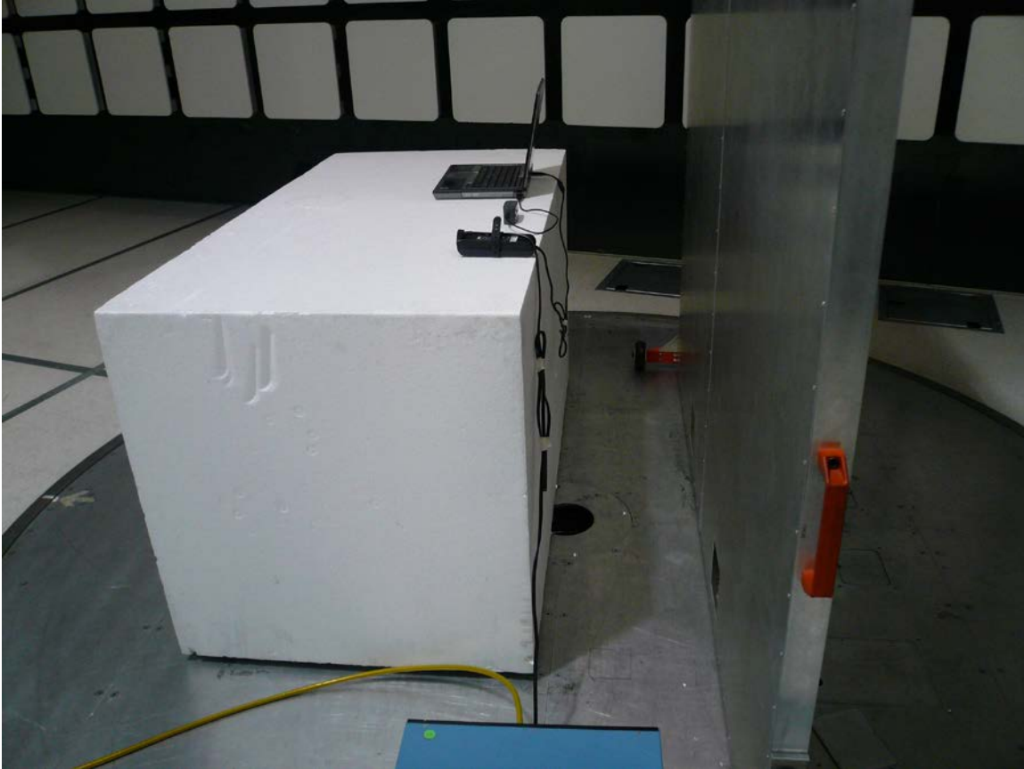
Figure 9: AC Conducted Emission Test Setup (Front)
