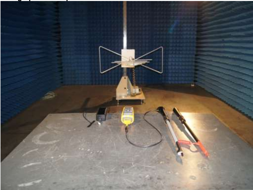
Photograph 2: Set-up for Radiated Emission – 30-1000 MHz
