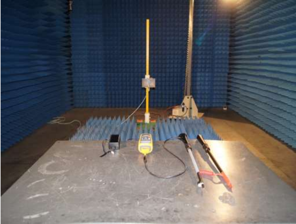
Photograph 3: Set-up for Radiated Emission – 1-18 GHz
