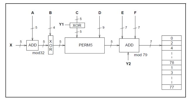
The X input determines the phase in the 32-hop segment, whereas Y1 and Y2 selects between master-to-slave and slave-to-master. The inputs A to D determine the ordering within the segment, the inputs E
