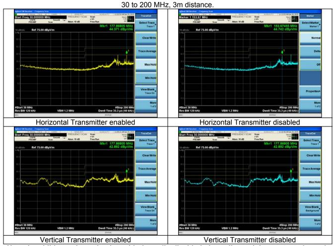
Note: In addition to investigation with the radio disabled, the radio module was tested standalone and confirms that emissions seen are not those of the radio module.
