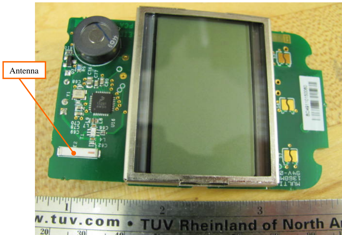
Figure 4: View display side of the PCB, also showing the transmitter section.
