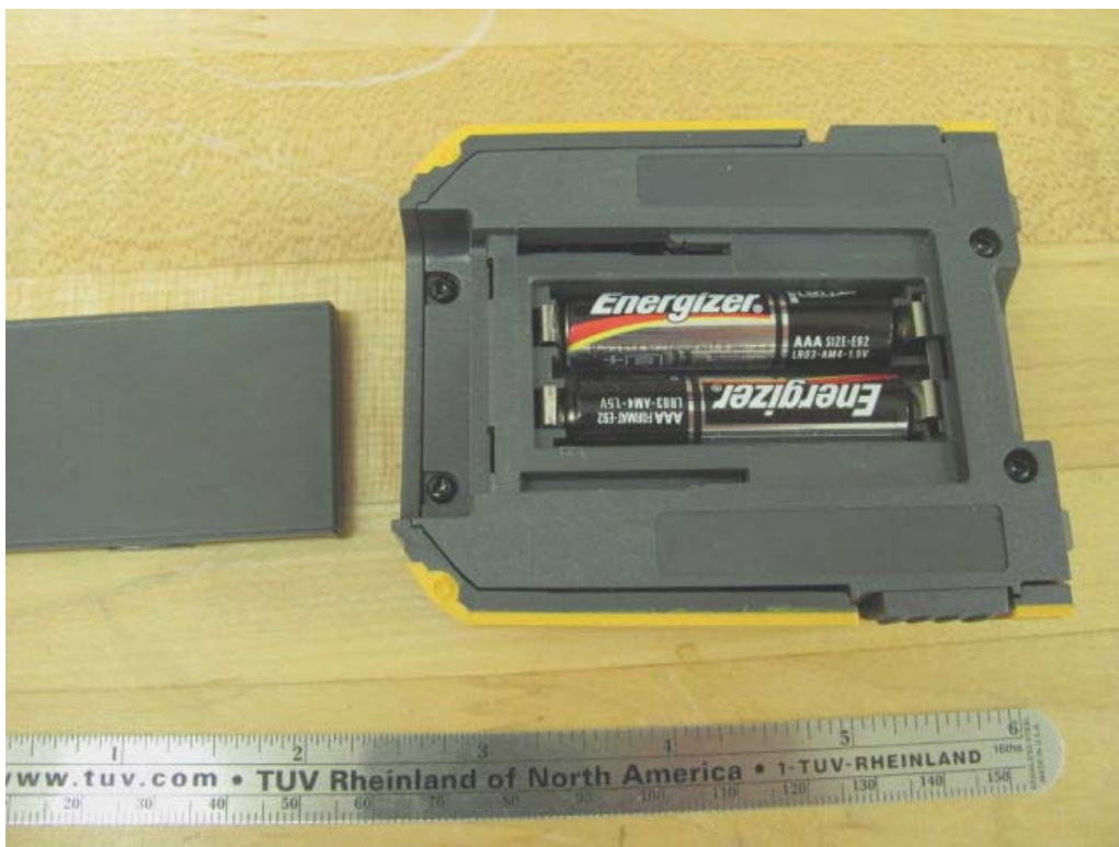
Figure 4: Rear view of display unit with battery compartment open
