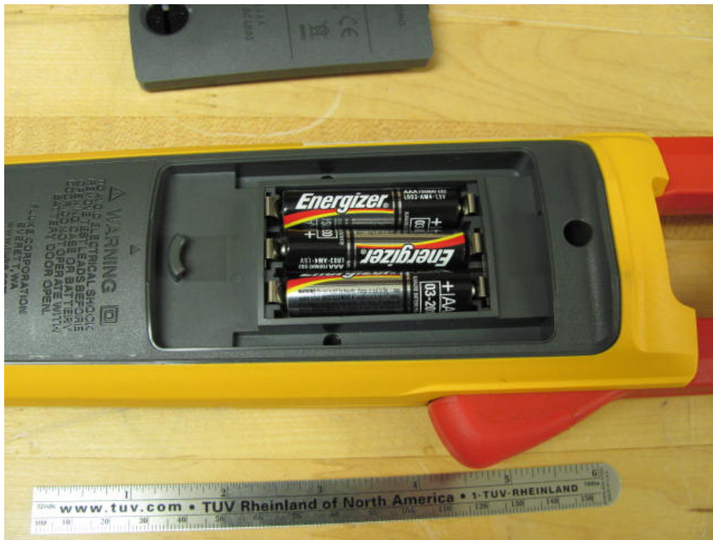
Figure 6: Bottom view of base unit with battery compartment open
